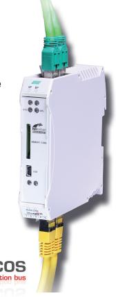
The gateway netTAP 151 transmits IO data bidirectionally between any two industrial Real-Time Ethernet networks. It is the ideal solution for installations with heterogeneous networks or such of the same kind to exchange data across given network boundaries. With more than 25 different combinations of the protocols PROFINET, EtherCAT, EtherNet/IP, POWERLINK, Sercos and Modbus TCP, the device series provides a solution for any conversion.
